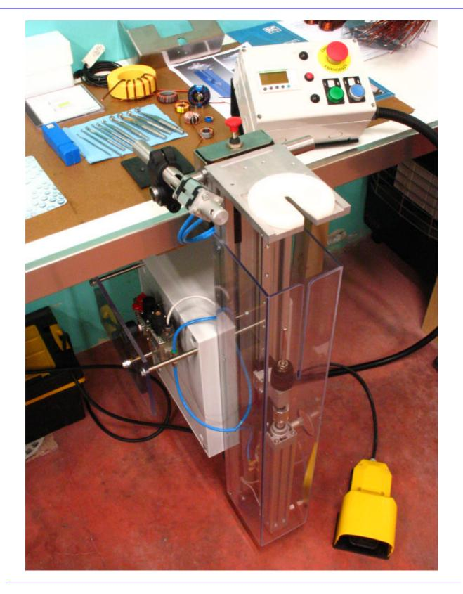
The semi-automatic toroidal coil winder has been designed, built and protected to wind spires of different kinds of copper wires on various typologies of ferromagnetic toroidal nucleus.
